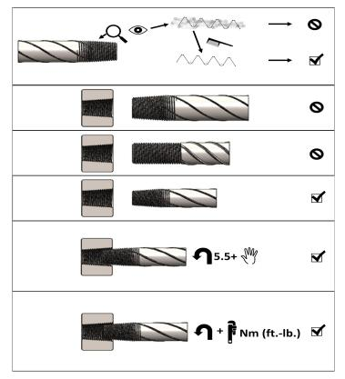
NOTE :Anchors must be assembled with calibrated torque wrench. Torque wrench must be calibrated at least every 24 months (+/- 15%).
